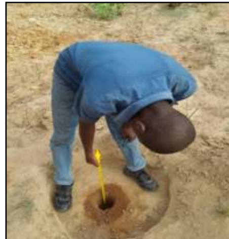
Figure 6. Measurement of water level drop
